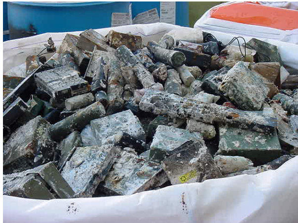
Figure 4: Batteries affected by the fire
