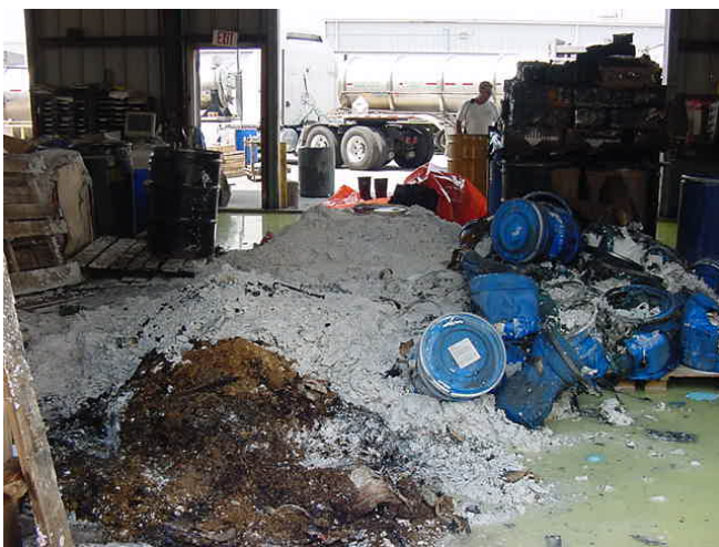
Figure 11: Fire started near sawdust pile, east side blue drums contain calcium hypochlorite
