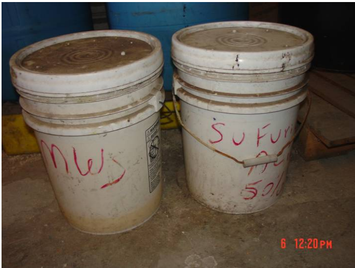
Figure 9: Improperly labeled, undated containers
