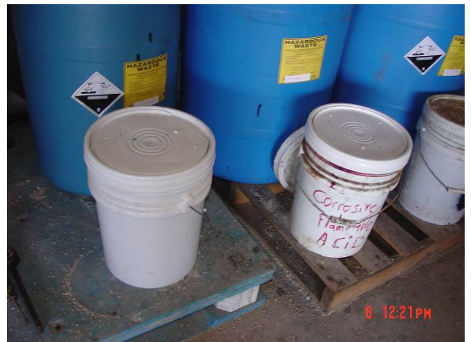
Figure 12: Improperly labeled, undated containers
