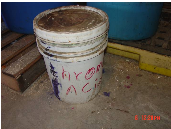
Figure 11: Improperly labeled, undated container
