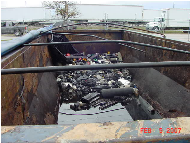
Fig. 5-Used oil filters, roll-off container is containment.
