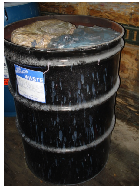
Figure 16: Drum of distillation bottoms from Figure 15
