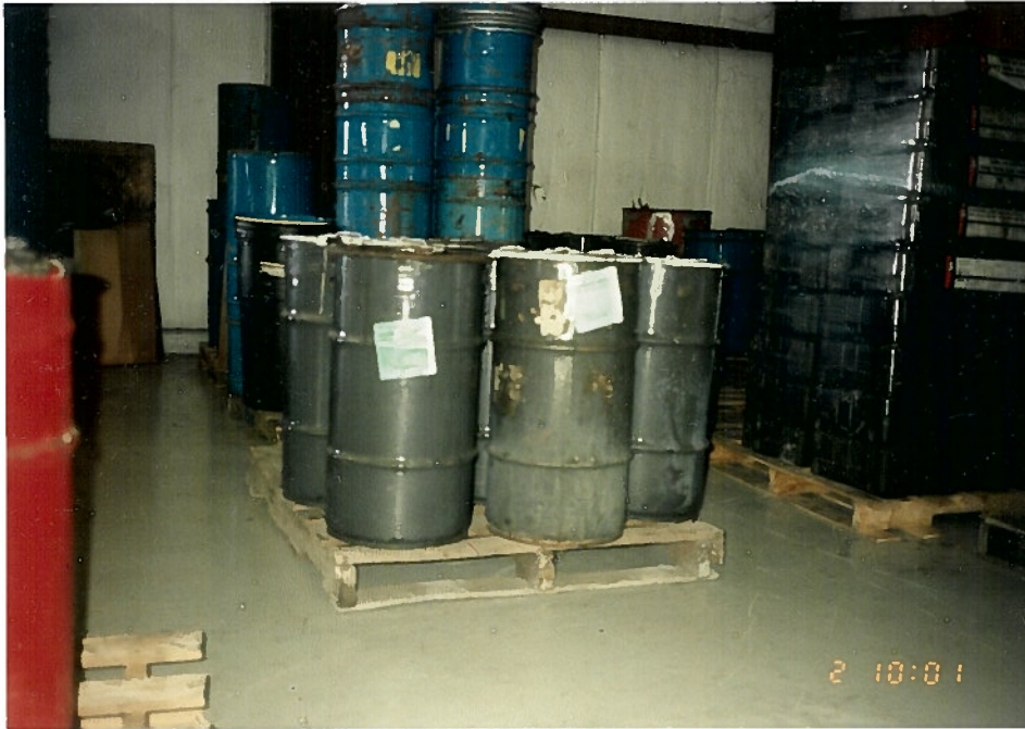
Photo 1c. Drums of waste within the Service Center Drum Storage Area (SWMU 1). The drums were positioned on wooden pallets and the epoxy-coated floor was in good condition. Note height of stacked waste drums.
