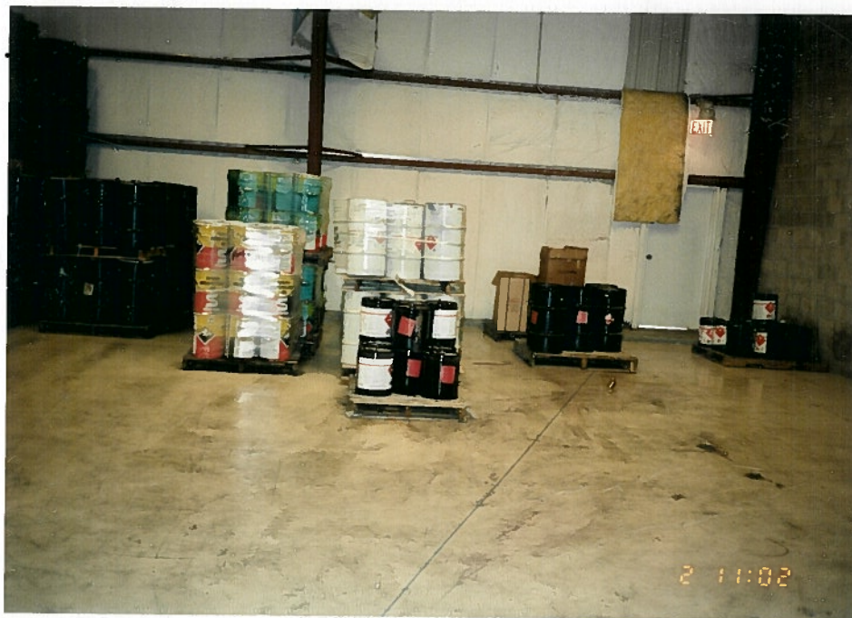
Photo 10a. The Drummed Flammable Waste Storage Room (SWMU 10). All drums were positioned on wooden pallets. Note that drummed waste to the left is stacked four drums high.
