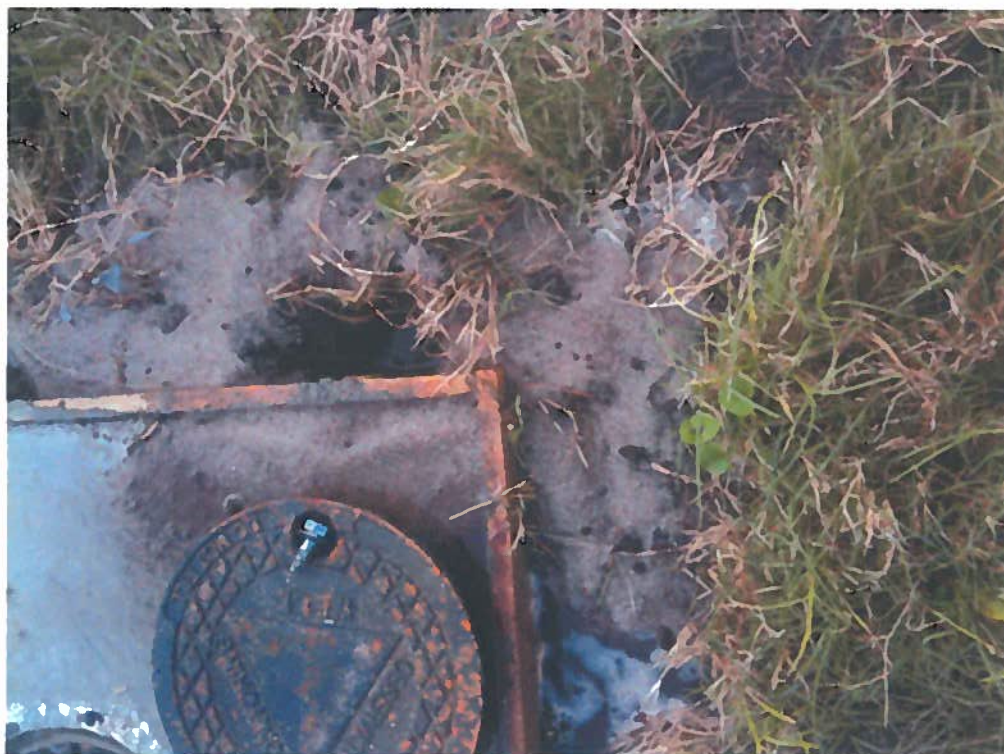
Monitoring well pad MW-2 right after septic tank water breached land surface bringing up monitoring well filter pack to land surface.
