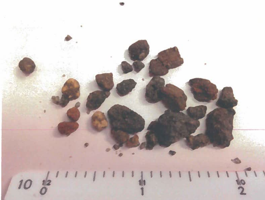
Rocks (possible hard pan) encountered in soil boring for MW-4 at five feet below land surface.
