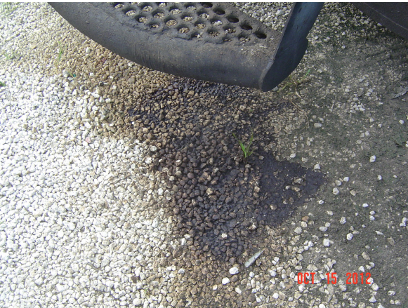
Photo 5 - oil leak under tanker
