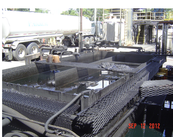
Photo 4 - oil in containment around used oil pit
