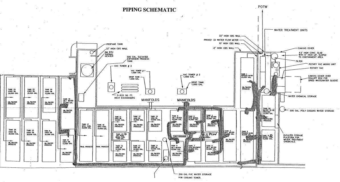
NOTE: WATER SIDE PIPING IS SHADED REMAINDER IS FOR OIL AND SPECIFICATION FUEL
