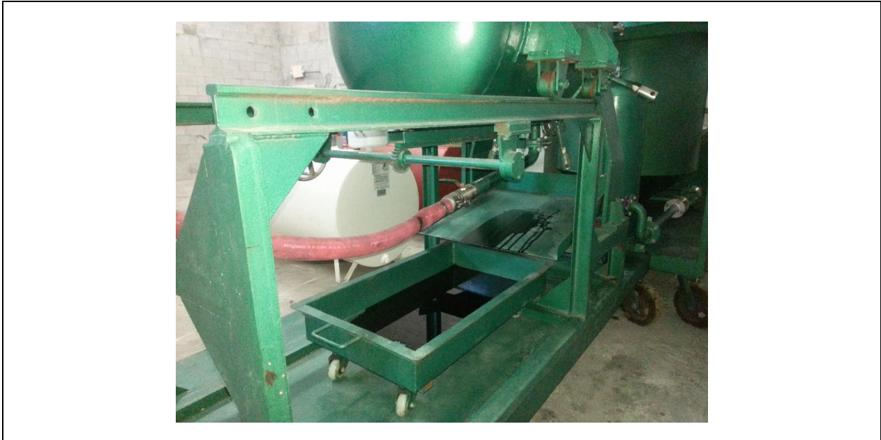
Description: Detailed view of the LYE-1000 Regeneration System Filter Press Tray for sludge collection
