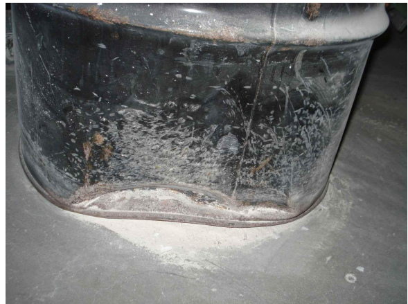
10. Damaged phosphor powder drum
