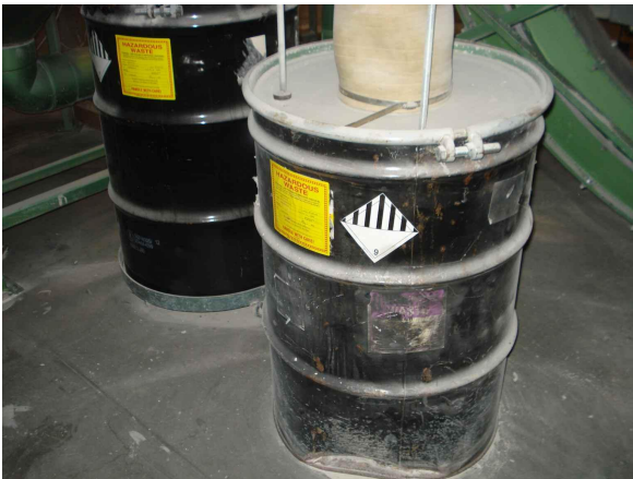
9. Drums collecting phosphor powder from filters
