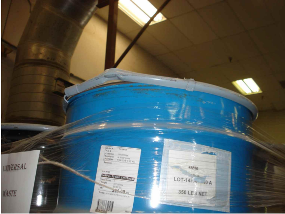
7. Crushed glass drum with damaged ring
