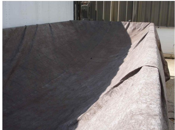
16. Tarp over processed glass container is not water tight
