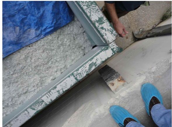
14. Processed glass container gate - not sealed
