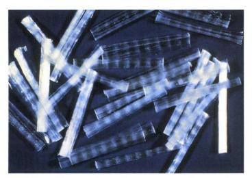
10. Groups of fibrillated fibers. The polypropylene fibers are fed into the concrete in fibrillated bundles in order to prevent balling during mixing. The mixing cycle breaks the bundles into idual fibers as shown in Illustration #12.
