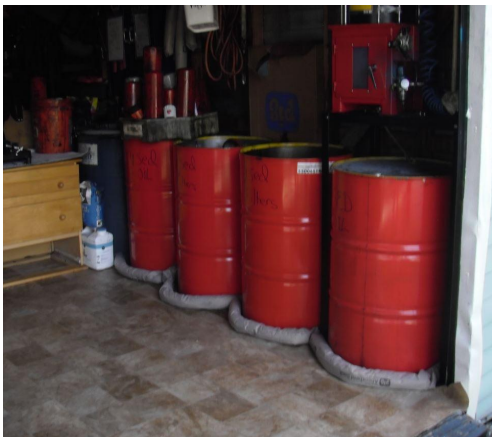
Drums without secondary containment.
