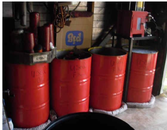
Drums without secondary containment.
