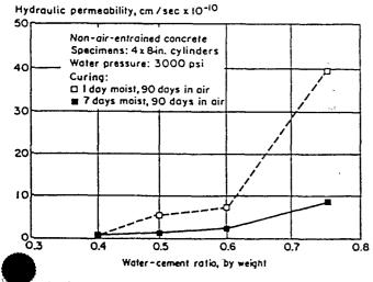
rig. 1-10. Relationship between hydraulic (water) permeability, water-cement ratio, and initial curing on concrete specimens. Reference PCA HM1170.
