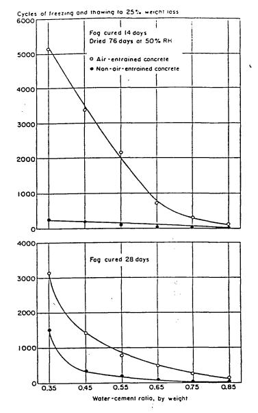
Fig. 1-9. Relationship between freeze-thaw resistance, water-cement ratio, and drying fcr air-entrained and nonair-entrained concretes made with Type I cement. High resistance to freezing and thawing is associated with entrained air, low water-cement ratio, and a drying period prior to freeze-thaw exposure. Reference 1-5.
