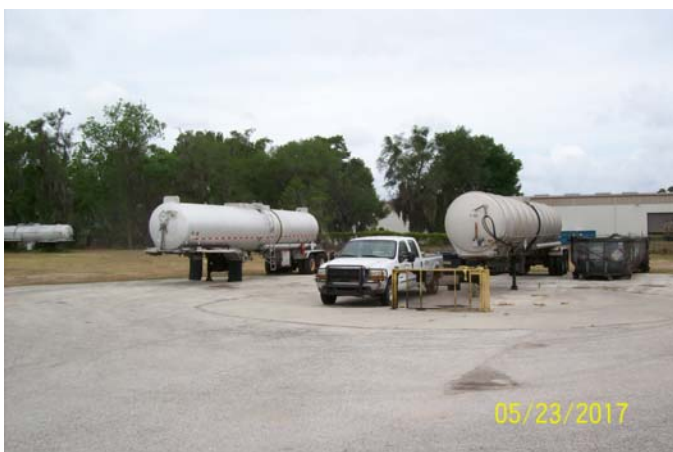
Photo ID # 101_0043: Tanker trailer T-45 on the left is empty; tanker trailer T-43 contained approximately 5,000-gallons of off-spec oil from the rail car; no containment.
