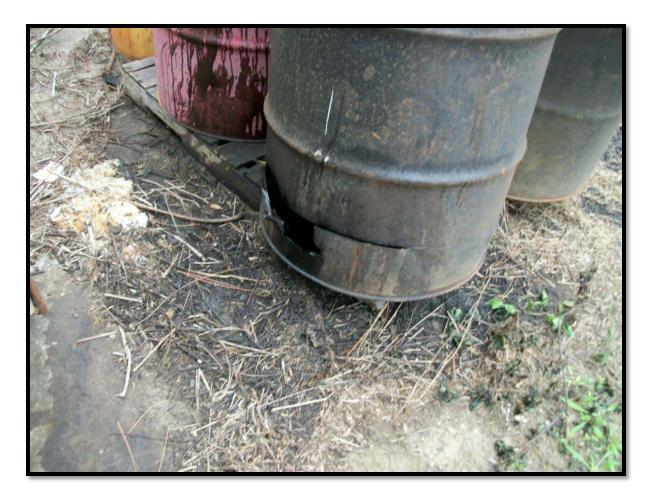
Not in secondary containment, bad condition, leaking, and it's unlabeled
