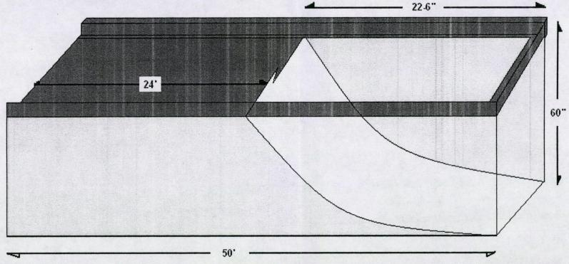
Bermed area surrounding bay is about 10" thick at the top, 16" tall and has a lip about 12" thick extending into the bay.
