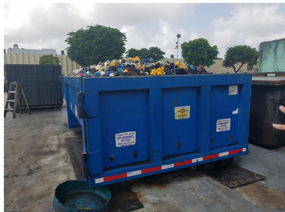
Drained Used Oil Filter Main Accumulation Container
