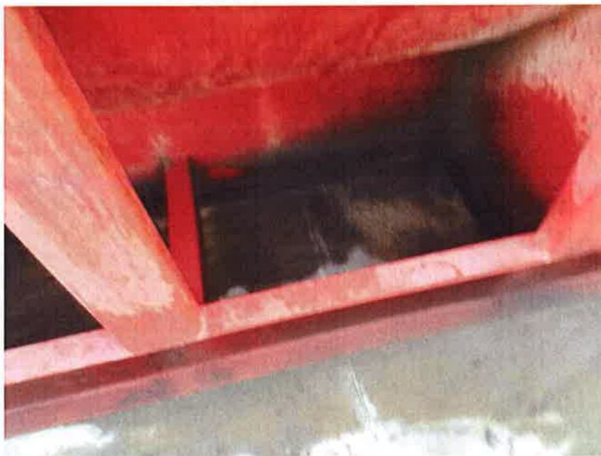
TYPICAL BRACING FOR TANK BOTTOM & SKID
