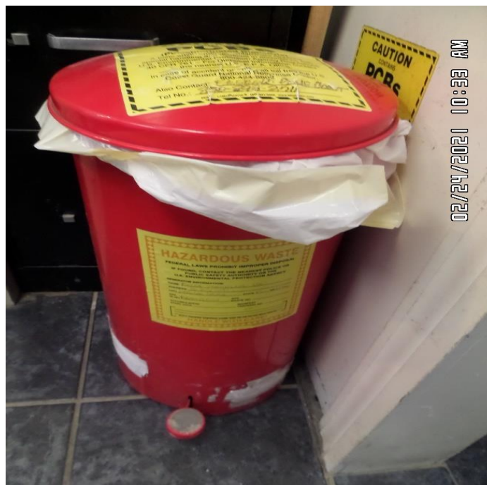
Figure 1 - Container storing PCB vials. The container did not have the hazard indication
