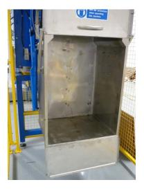
A drum can now be loaded. Alternatively the bottom door can be kept closed to allow smaller lamps and bulbs to be loaded loosely.
