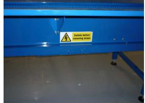
End panel of flatbed conveyor should be removed monthly and any debris cleaned from under the belts.
