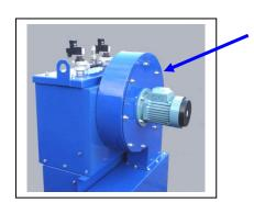
Remove the nuts securing the motor mounting plate to the fan case.
