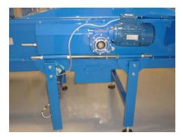
Flat plate drawers under both flatbed conveyors should be removed every week
