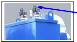
Each valve is fitted with an individual timer. The timer has two adjustable controls. The duration control marked "ms" should always be set to 100. The other marked "min" is the time between pulses and may be set to suit conditions, but not less than 0.5 minutes.
