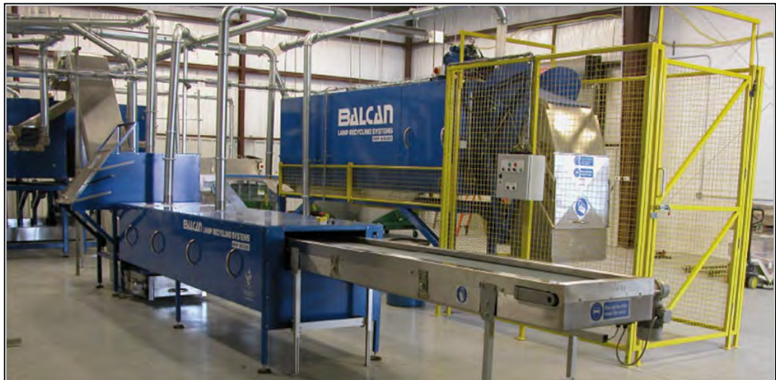
Photo Inset No. 9: Section 1 - Primary Process Unit in foreground; Section 2 -Secondary Process Unit to the right; and Section 3 - Cleaning/Sorting Unit at far backend.
