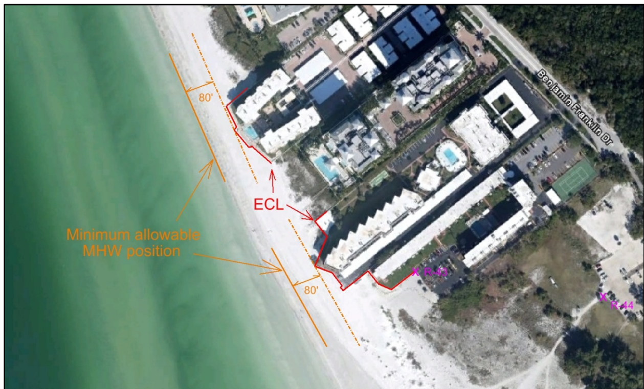
Figure 3. Minimum required shoreline positions along southern Lido Key.
