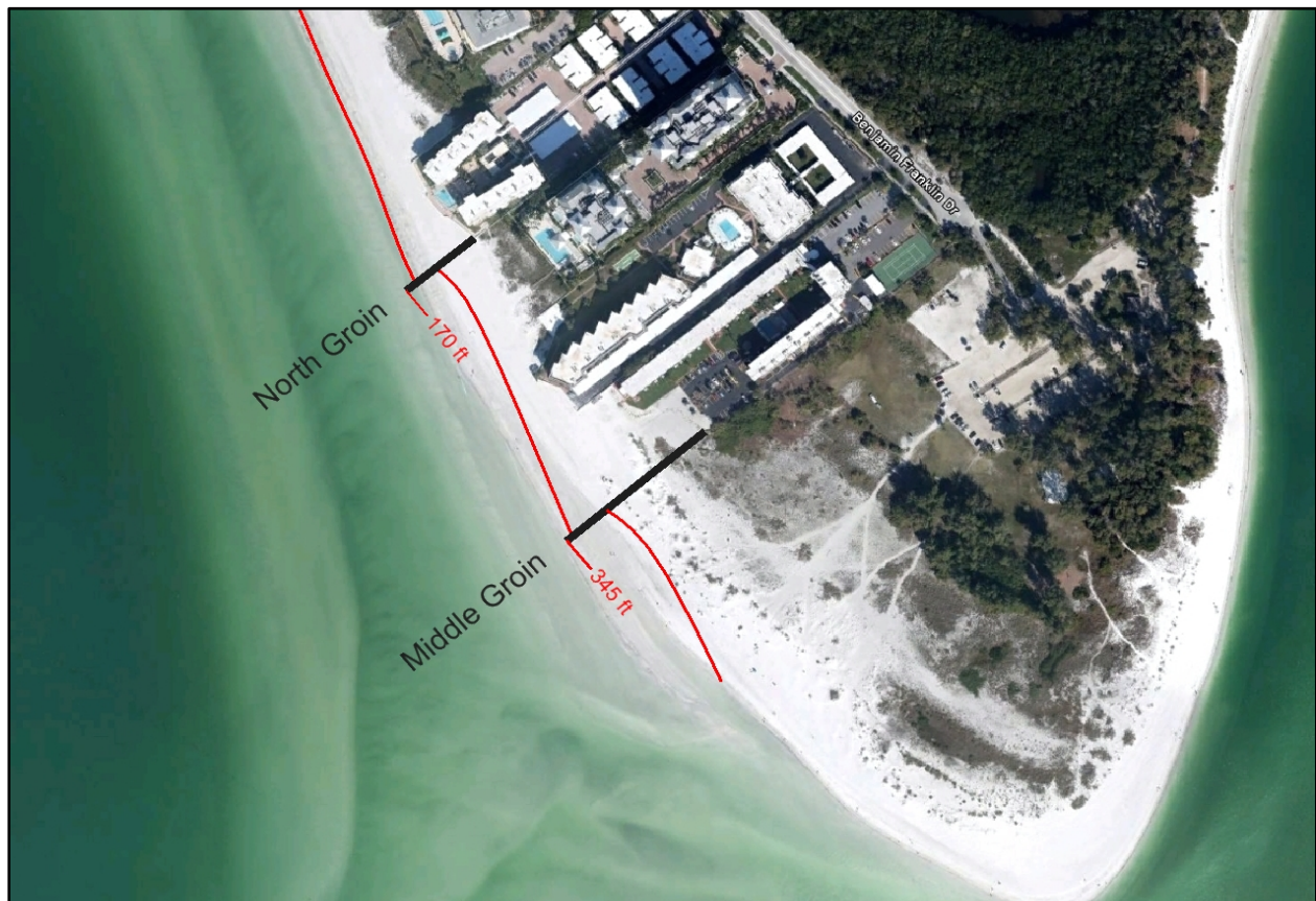
Figure 7. Calculated final equilibrated shoreline positions.
