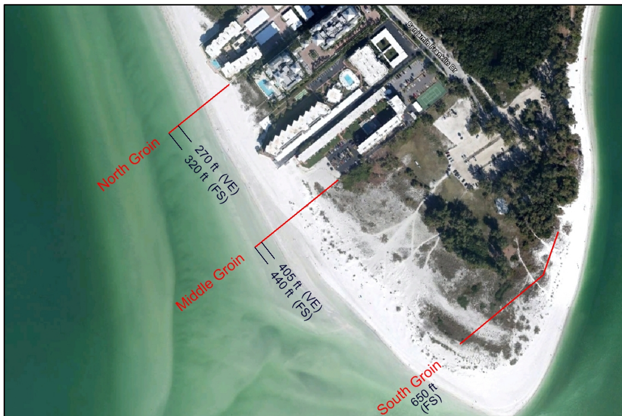
Figure 1. South Lido Key groin field. Recommended structure lengths from the Feasibility Study (FS) and Value Engineering Study (VE).
