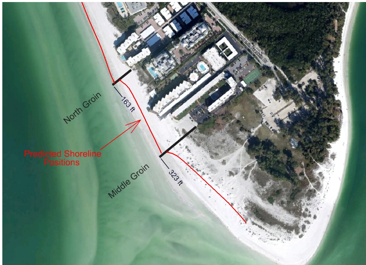
Figure 5. Predicted groin lengths and shoreline positions resulting from the Case Study.
