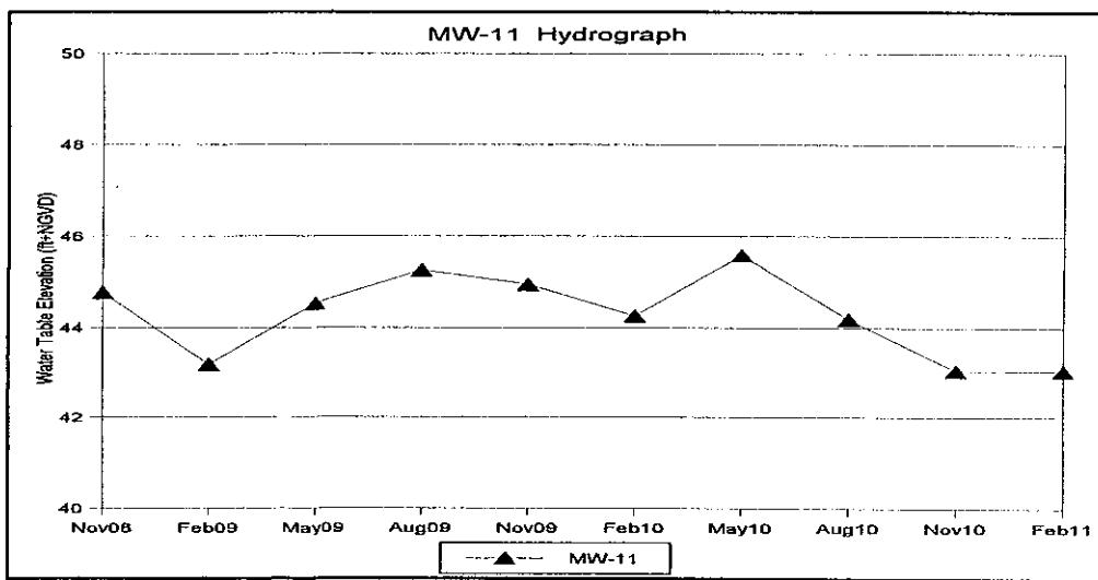
**MW-8, MW-10 and MW-11 Hydrographs**
