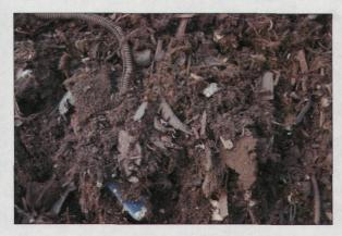
Close-up view of material in the final waste bunker (Fluff).
