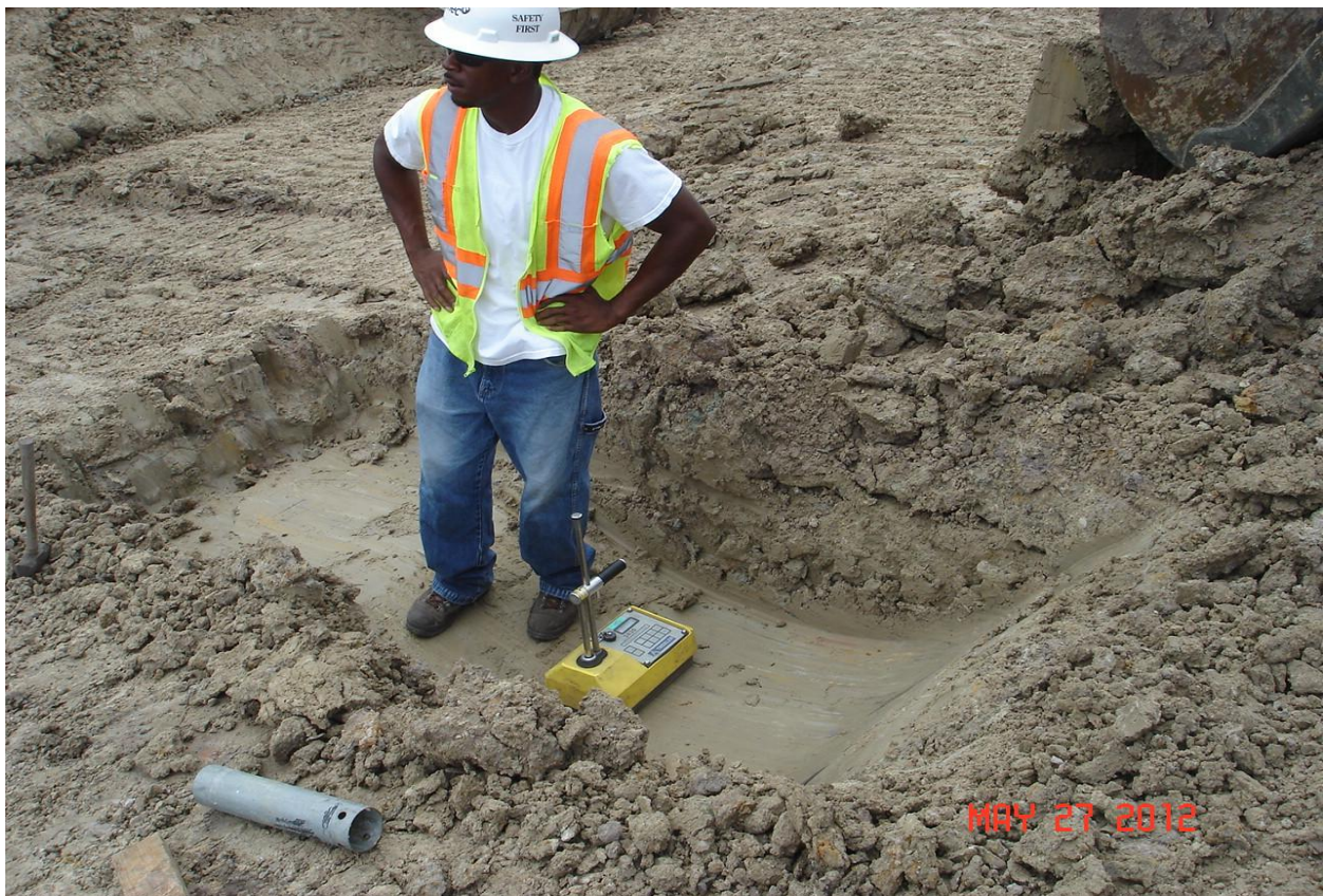
Density Testing Clay Downcomer D-27 (Phase I)
