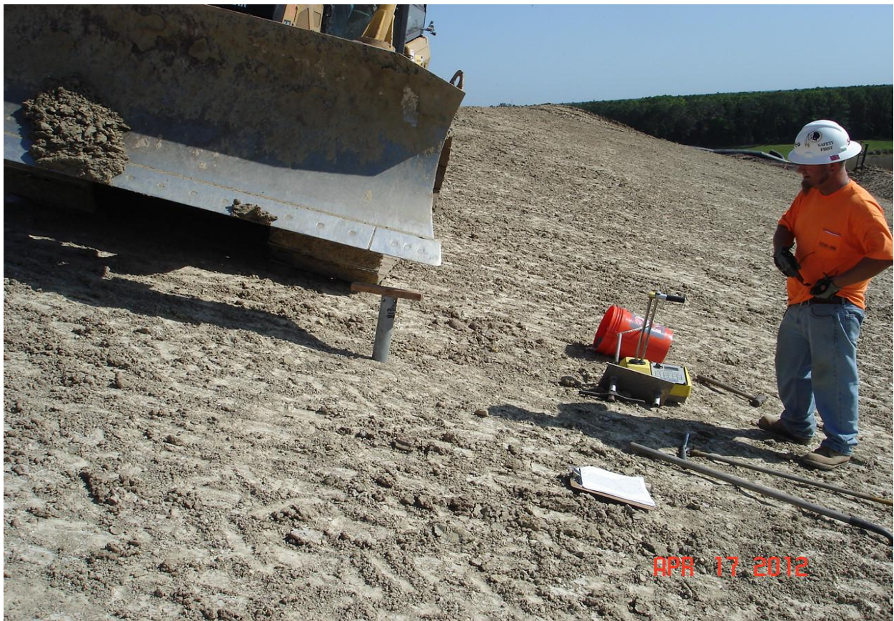
Pushing Shelby Tube for Permeability Test – Phase I
