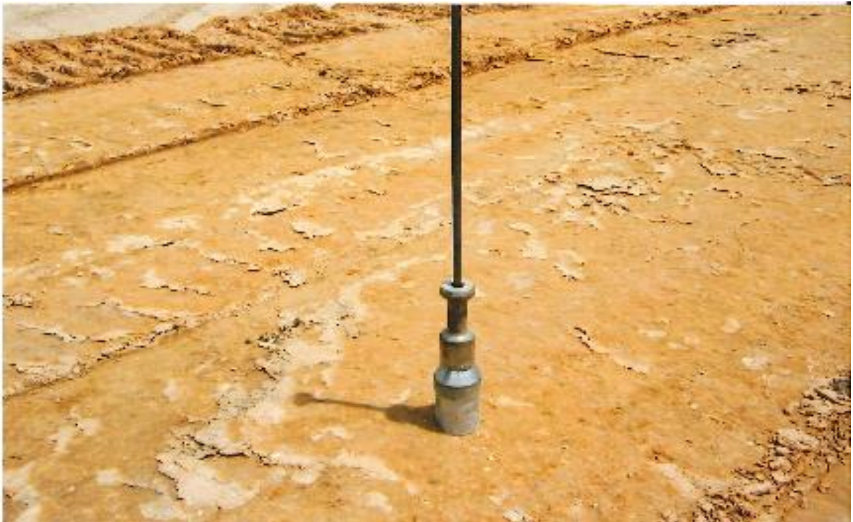
Moisture Density Test was performed using the drive cylinder.
