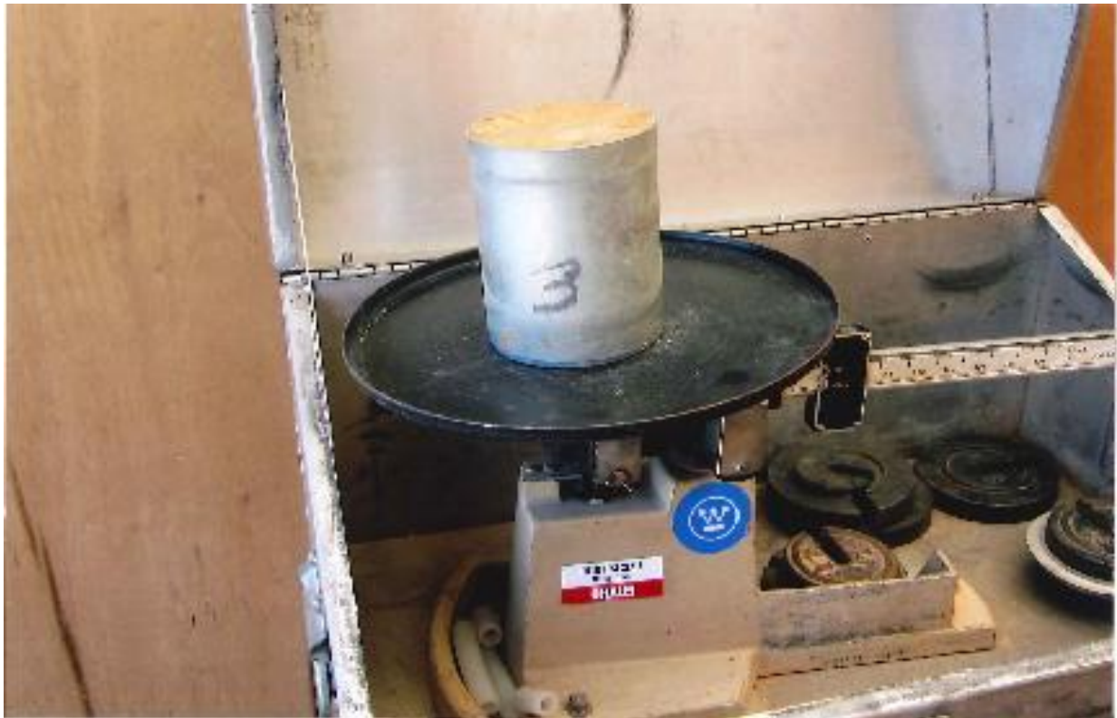
Drive cylinder being weighed in the field laboratory.
