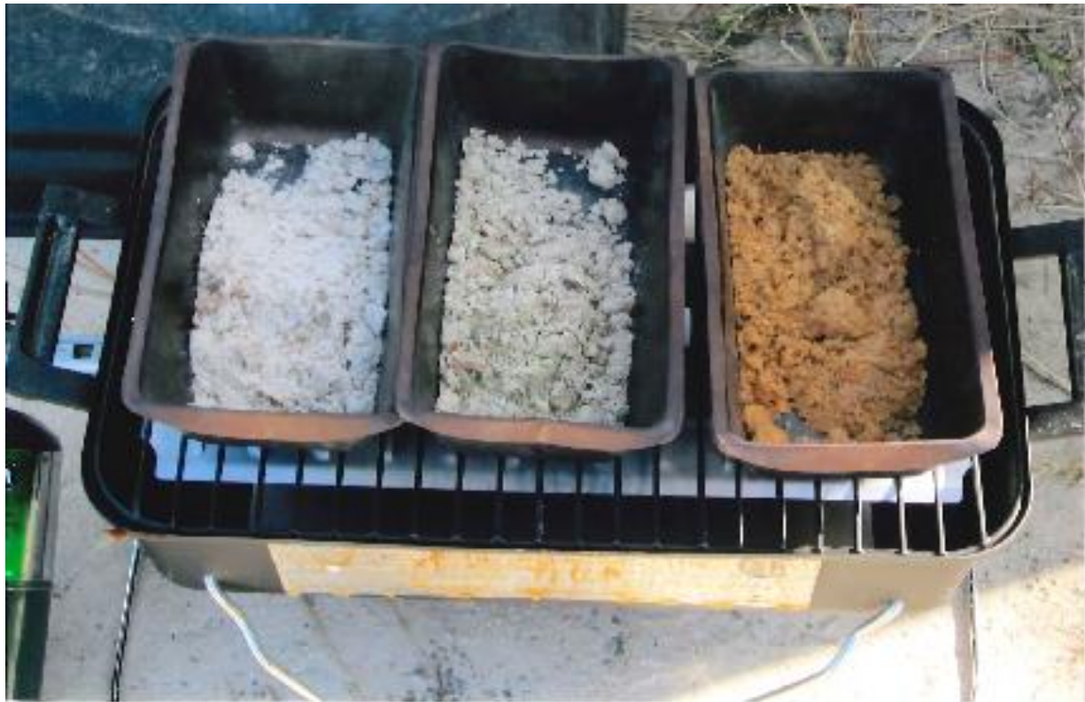
An oven was used to dry samples for moisture test.
