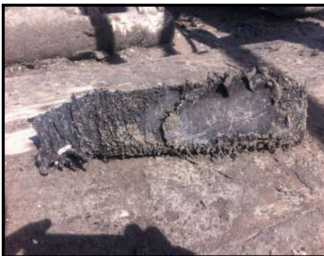
Photograph 9: Debris Plug/Rubber Tire (extracted from casing)
