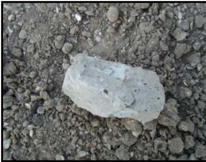
Photograph 7: Typical Consolidated Clay with Phosphates Plug (extracted from casing)
