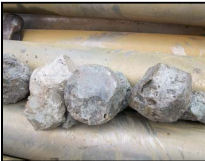
Photograph 8: Typical Limestone/Rock Plugs (extracted from casing)
