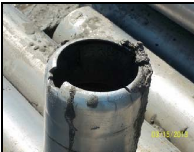
Photograph 12: Typical View of Worn Bit
