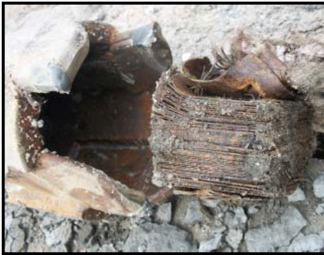
Photograph 10: Debris Plug/Rubber Tire (extracted from casing)
