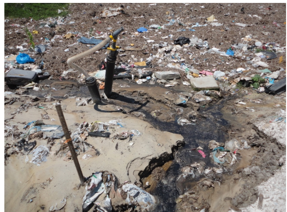
Leachate and Exposed Waste
