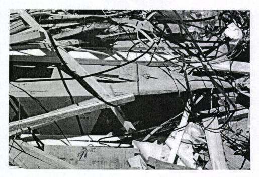
This load is from a construction company that builds trusses and floor joists. It contains treated wood. Green colored sawn boards are treated. Other sawn boars may be untreated. Additional testing may be needed to confirm treatment.
