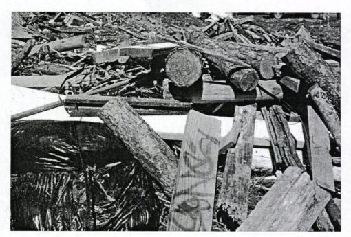
This load is a mix of yard waste, CCA-treated fencing and CCA-treated landscaping timbers. Treated wood can be identified based on the fact that it is sawn and is characterized by a green hue. The sawn board in the bottom is obviously treated. It is difficult to tell for the highly weathered sawn boards.
