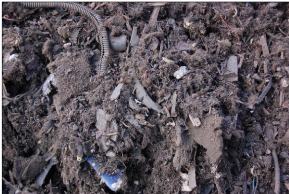
Close-up view of material in the final waste bunker (Fluff).
