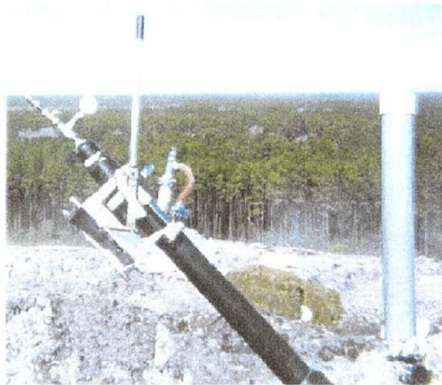
Pressure testing of header line.
