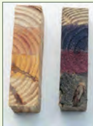
Stain effects on untreated wood (left) and treated wood (right).
