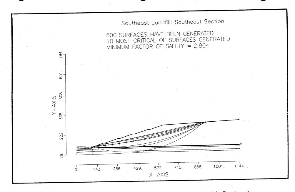
Figure 20A - Circular Arc Analysis with Replaced Fill Sand in Stratum I (Deep Failures)
