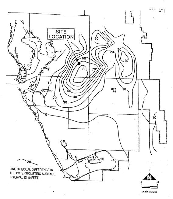
NOTE: NEGATIVE VALUES INDICATE A HIGHER POTENTIOMETRIC SURFACE IN THE UPPER FLORIDAN AQUIFER THAN THE INTERMEDIATE AQUIFER. CONTOURS ARE BASED UPON AN AVERAGE OF MAY AND SEPTEMBER USGS POTENTIOMETRIC SURFACE MAPS FOR EACH AQUIFER SYSTEM.
