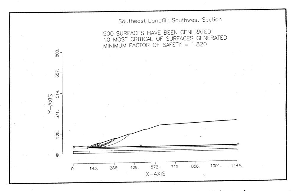
Figure 18B - Circular Arc Analysis with Replaced Fill Sand in Stratum I (Shallow Failures)
