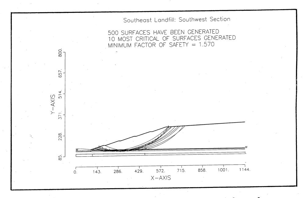
Figure 17A - Circular Arc Analysis with Phosphatic Waste Clay in Stratum I
