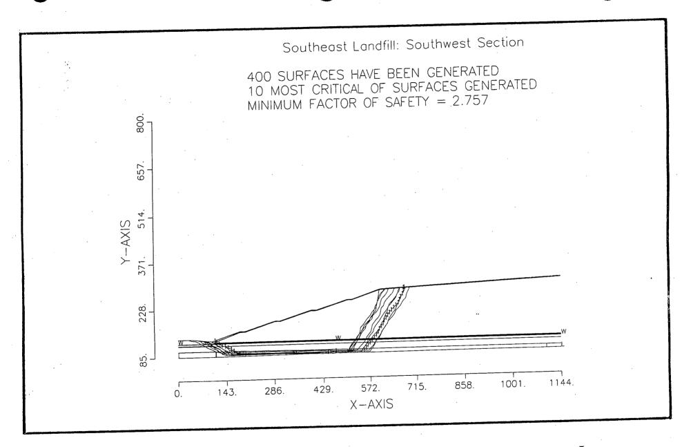
Figure 19A - Sliding Block Analysis with Replaced Fill Sand in Stratum I (Deep Failures)
