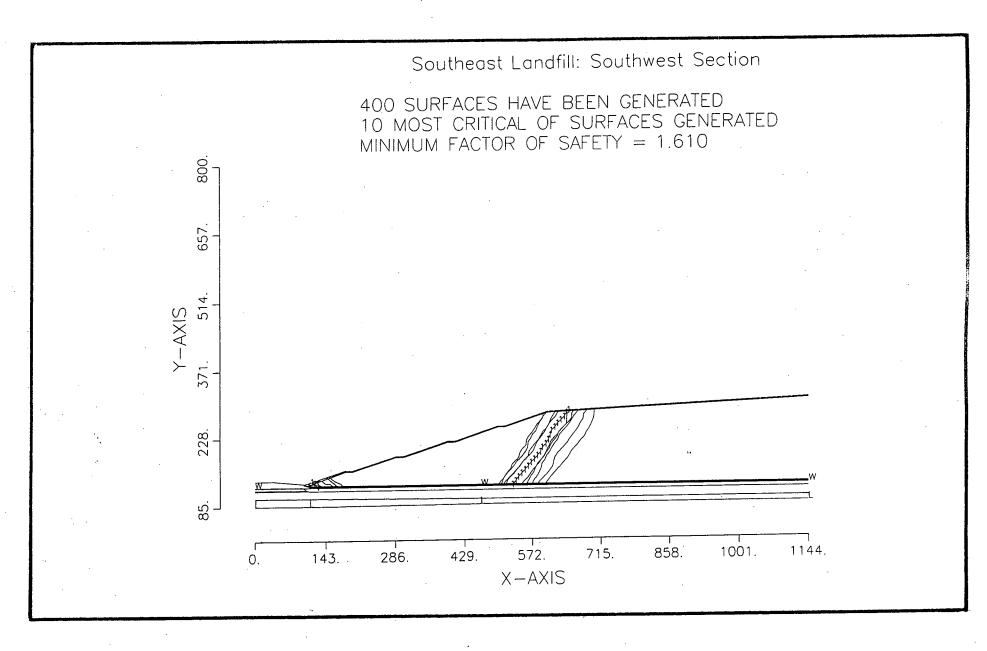
Figure 19B - Sliding Block Analysis with Replaced Fill Sand in Stratum I (Shallow Failures)
