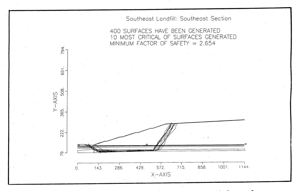
Figure 21A - Sliding Block Analysis with Replaced Fill Sand in Stratum I (Deep Failures)
