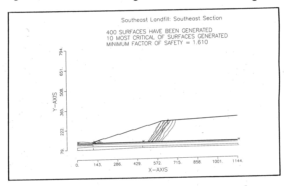
Figure 21B - Sliding Block Analysis with Replaced Fill Sand in Stratum I (Shallow Failures)
