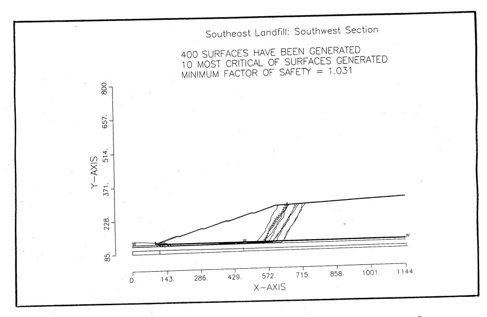
Figure 17B - Sliding Block Analysis with Phosphatic Waste Clay in Stratum I
