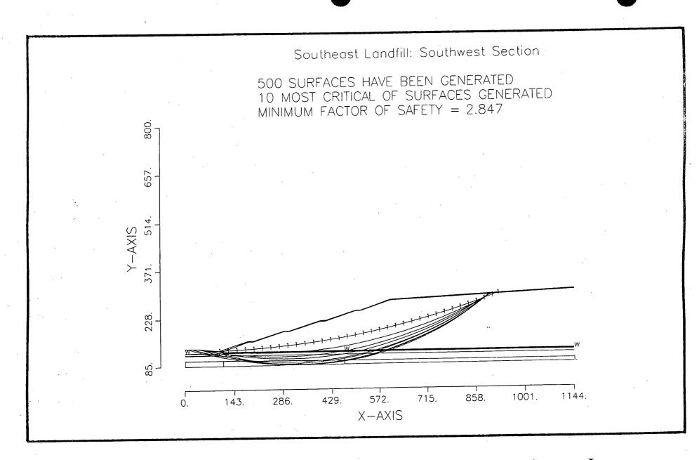
Figure 18A - Circular Arc Analysis with Replaced Fill Sand in Stratum I (Deep Failures)
