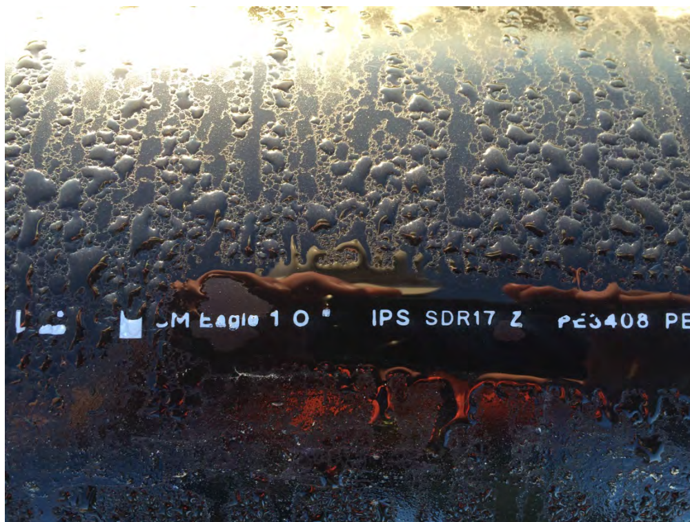
Photograph 20: 10-in. SDR 17 HDPE Pipe (used during horizontal collector construction).
