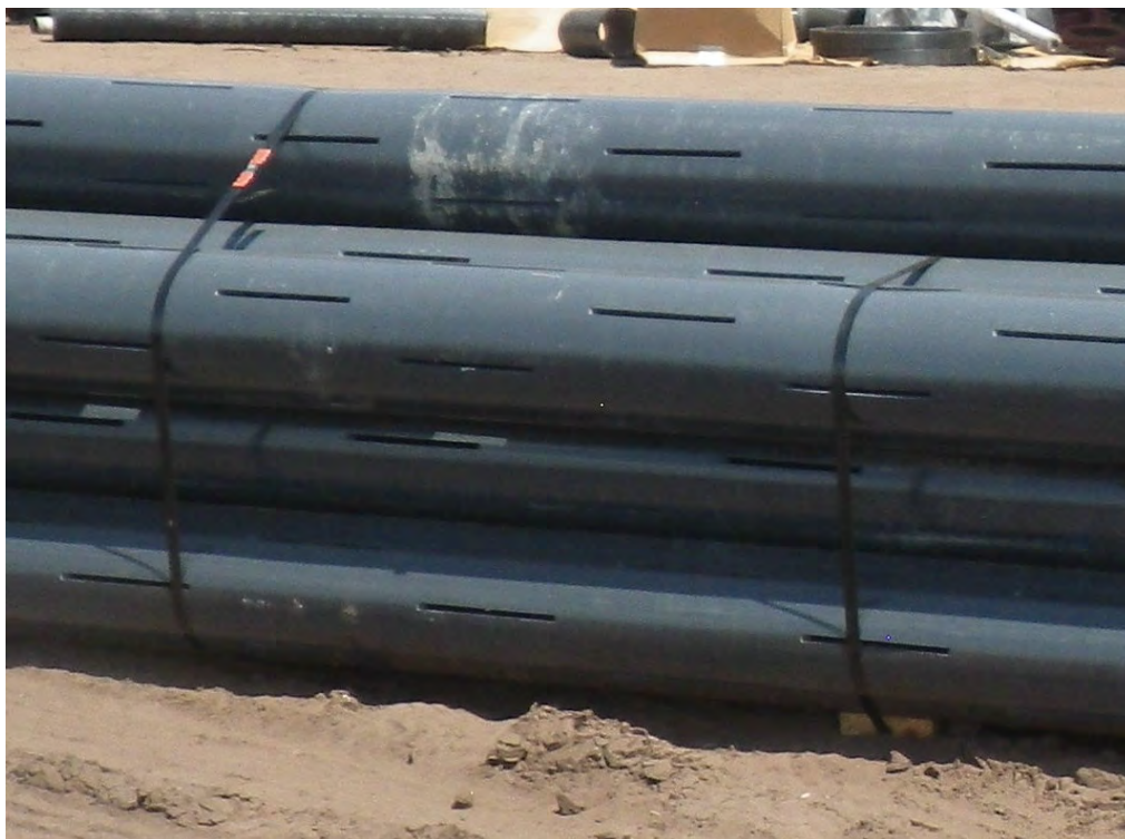
Photograph 3: 8" SCH 80 PVC 45° apart, staggered rows.
