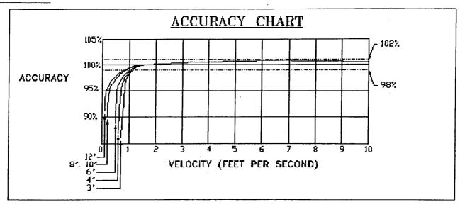
Standard flowrates for McCrometer propeller meters are shown below. Readings are guaranteed accurate within  $\pm 2\%$  in these flowrates. Please note that over 80 percent of the meter's flow range, the accuracy is better than  $\pm 1\%$ .
