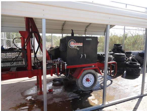
Shearer used for cutting tires
