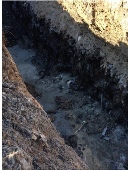
Phase II trench “B” looking south showing top of sand layer.
