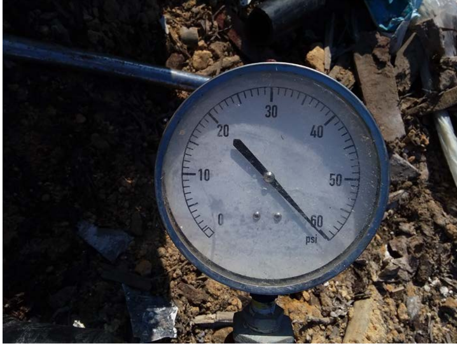
(Photograph 35: Passing 2" air and forcemain air test)
