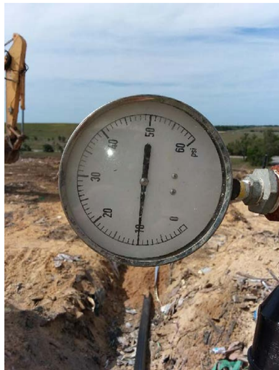
(Photograph 54: Passing 8" header and 6" lateral air test on northside)
