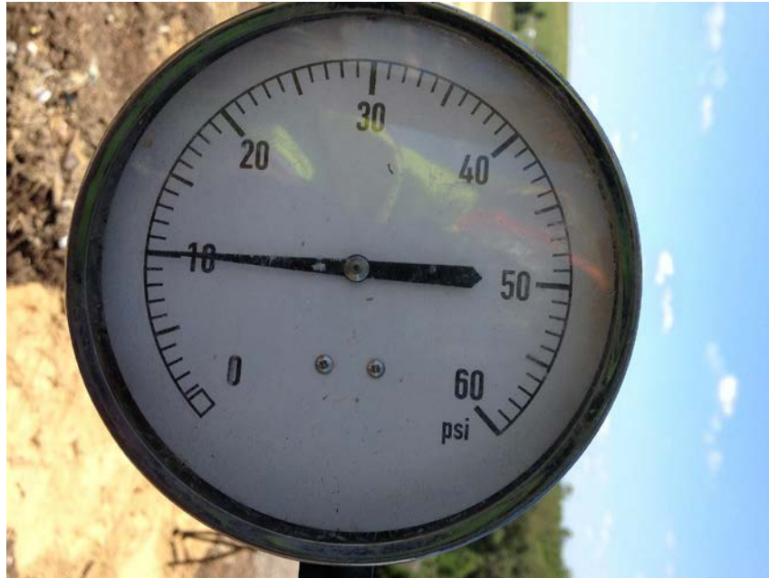
(Photograph 37: Passing 8" header and 6" laterals air test on northside and eastside)
