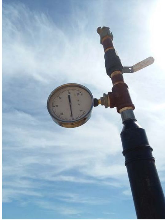
(Photograph 31: Passing air test for 8" header and 6" lateral)
