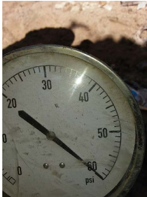
(Photograph 42: Passing 2" air and 2" forcemain air test on southside)
