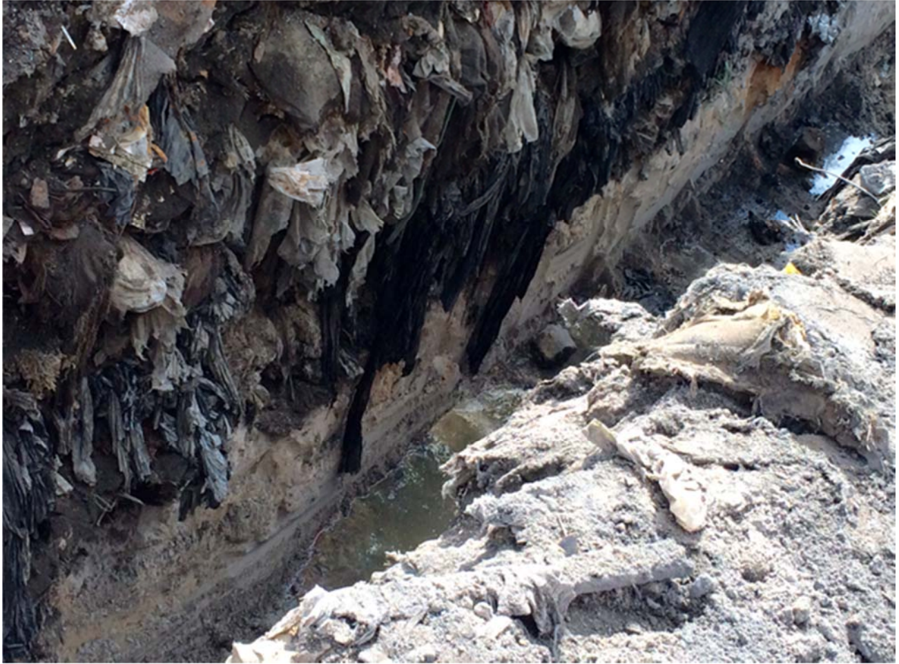
Figure 5-3. Looking down the trench in the section closest to the piezometer. The sidewall of the trench shows the 4-foot sand layer at the bottom with MSW on top of it. Note the heterogeneity in the MSW layer. When this section of the landfill was excavated, the sand was originally reported to be dry. However, water soon began to seep from the side wall, where the black agricultural plastic is located (the water did not originate in the sand layer). The water ponded at the bottom of the trench, as can be seen in the figure above.
