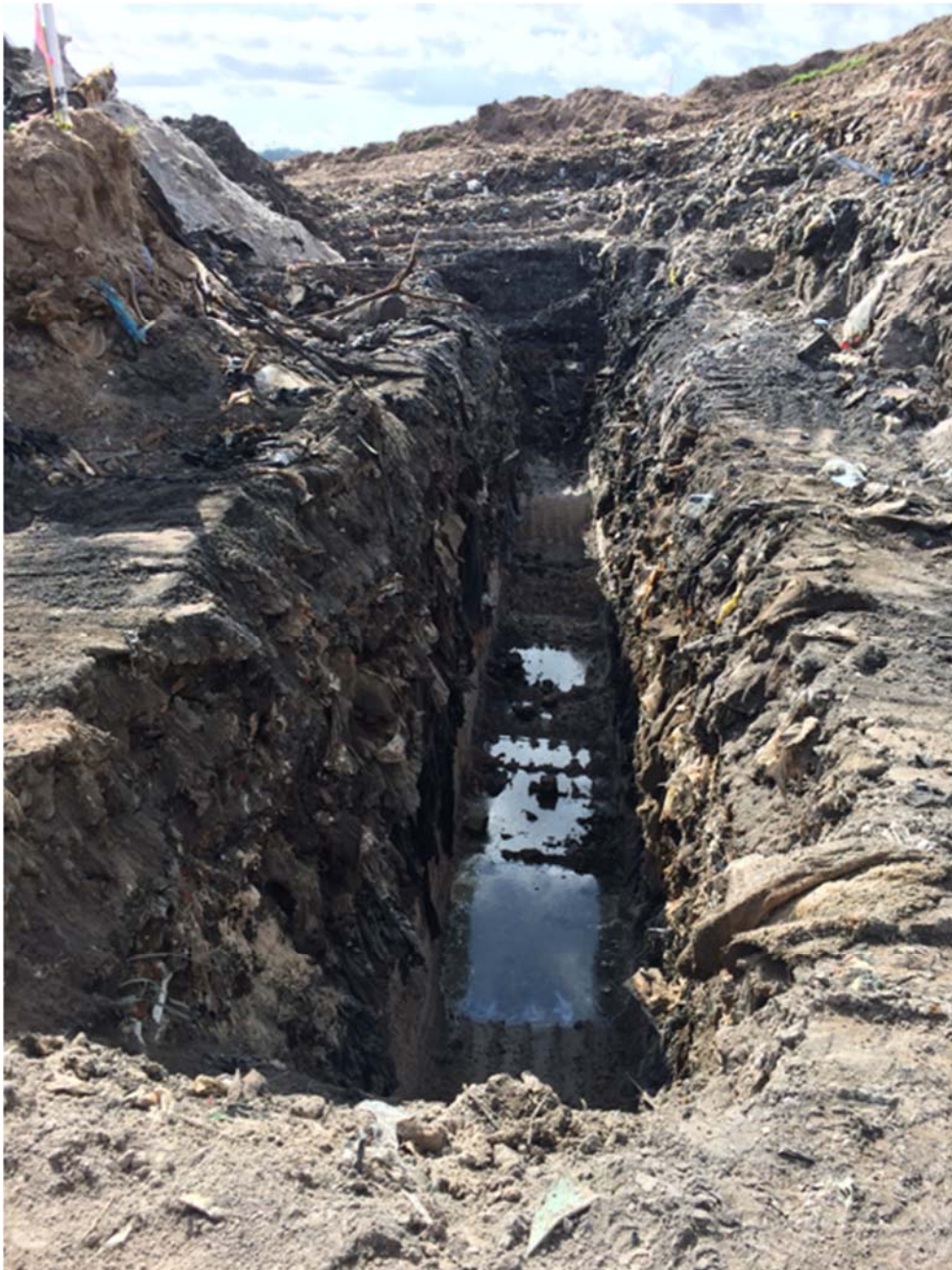
Figure 5-1. Trench dug near piezometer SB-32 on April 26, 2018. The piezometer is shown in the top left hand corner of the picture. The sand drainage layer was initially dry when it was excavated. A significant buildup of leachate occurred when the section of the trench nearest to the piezometer was dug up. This leachate originated from the middle layers of the MSW, not the sand drainage layer. About 0.4 feet of leachate developed in that area of the trench.
