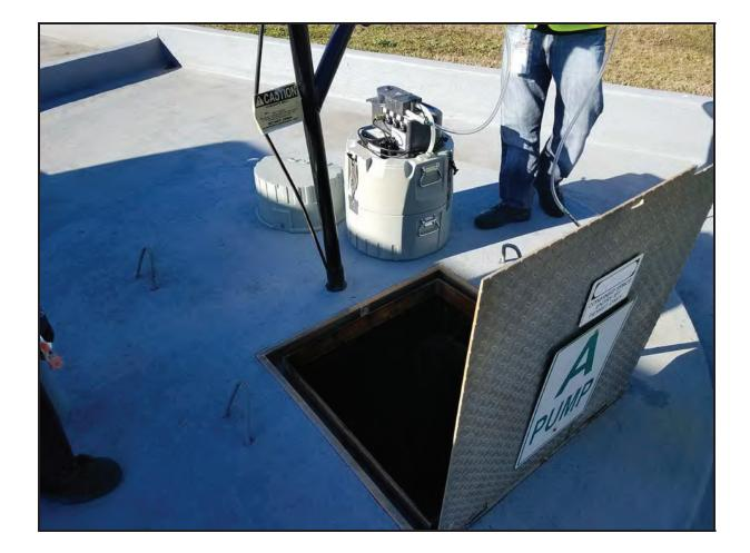
Photograph 1. Auto-Sampler Setup on Pump Station A (PS-A)
