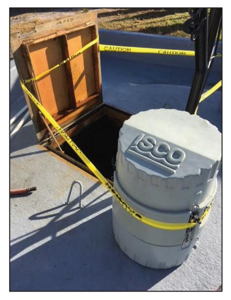
Photograph 1. Auto-Sampler Setup on Pump Station A (PS-A)
