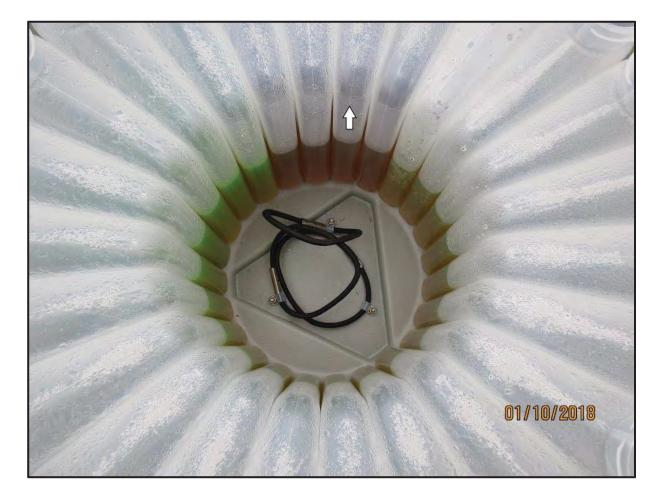
**Photograph 12.** Auto-Sampler Device Samples for the First 24 Hours (01/09/2018 - 01/10/2018). Arrow Indicates the 01/09/2018 12:00 p.m. Sample (Second Sample) and Advances Counter-Clockwise at One Sample per Hour. The 11:00 a.m. Sample (First Sample) is Directly to the Right of the Arrow.
