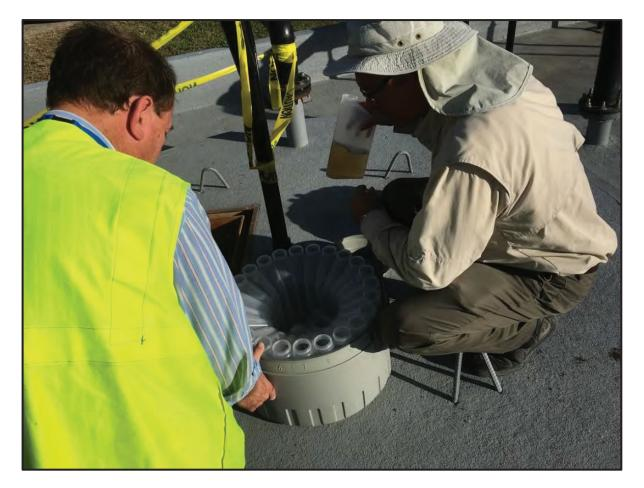
Photograph 10. SWMD Collects Sample 1 (1:00 p.m.), 2 (2:00 p.m.), and 3 (3:00 p.m.) from the Auto-Sampler for Laboratory Analysis
