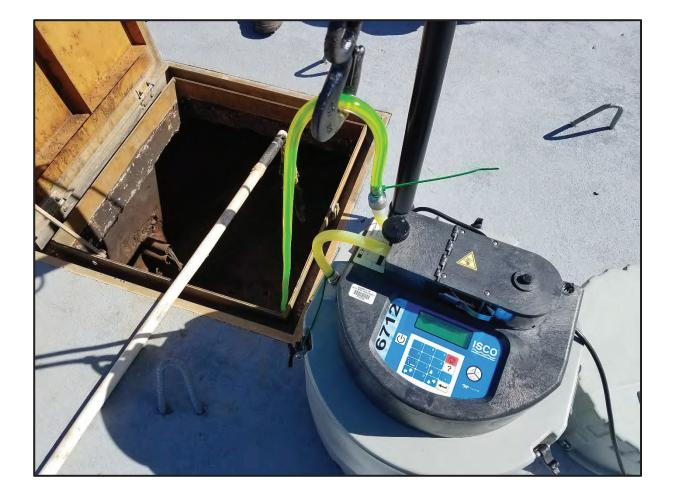
Photograph 9. 1:00 p.m. Check on Auto-Sampler at PS-A – Observable Fluorescent Dye
