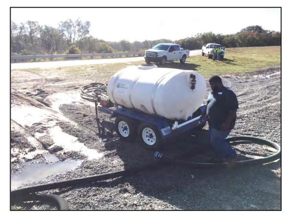
Photograph 3. 1,000 Gallon Portable Tank Used to Mix Water and Dye
