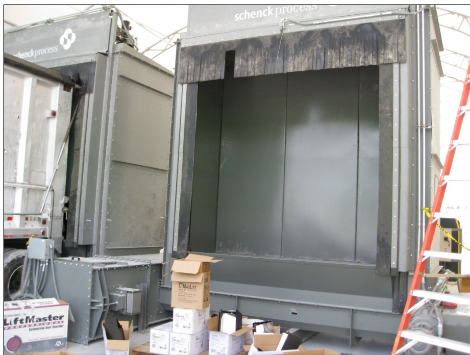
Photo 2. Two offloading docks of typical feeder system
