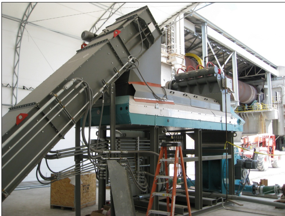
Photo 4. Typical Conveyors coming from offloading ports to metering system
