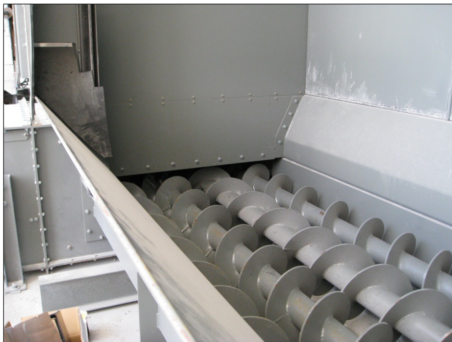
Photo 3. Typical screw conveyor in bottom of offloading ports
