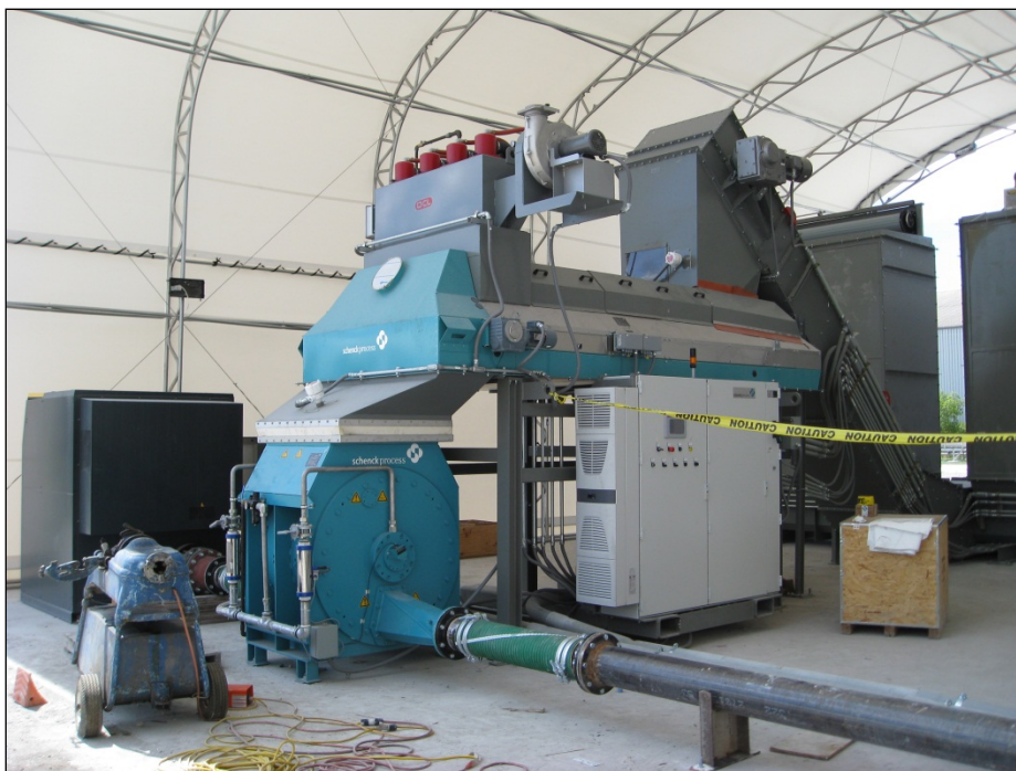
Photo 5. Typical Pneumatic blower from metering system to injection porthole
