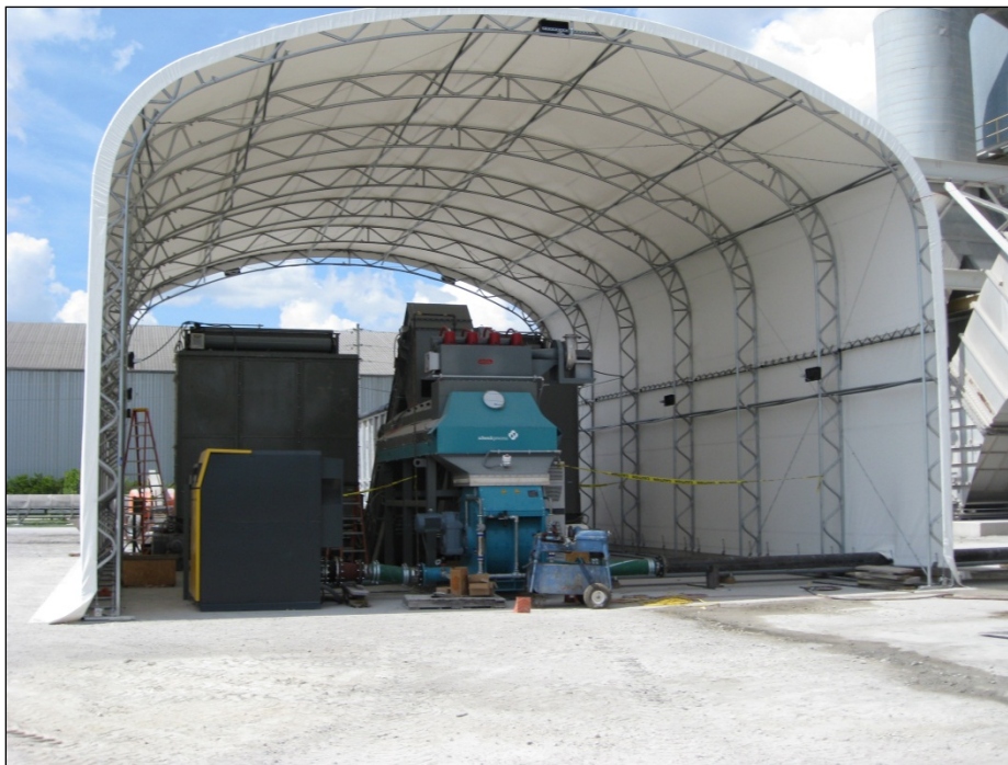
Photo 1. A typical covered feeder system
