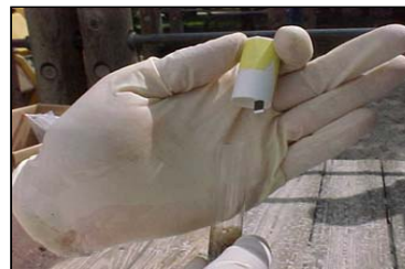
Positive arsenic test kit result shown by the dark brown spot on the test strip
