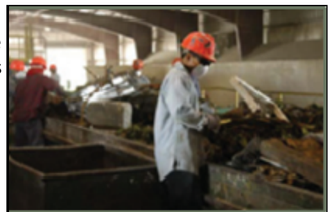
Recycling at Materials Recovery Facility emphasizing the process for wood sorting
