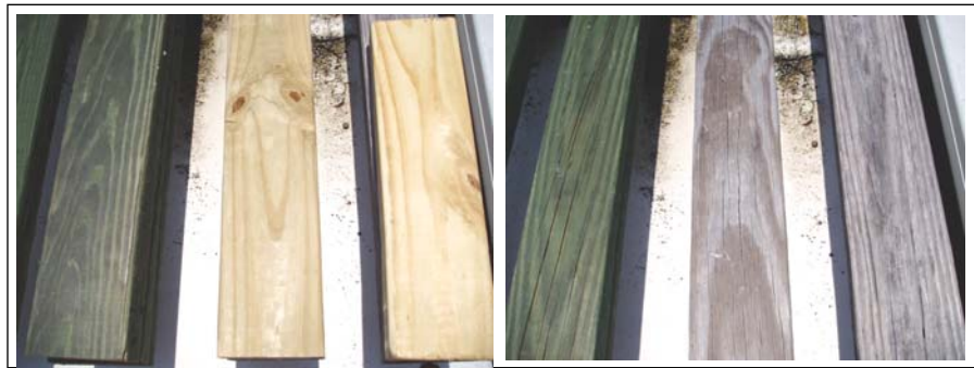
Color of New and Weathered CCA-Treated Wood
