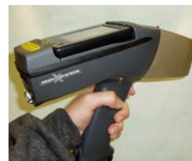
XRF unit for analyzing wood in the field
