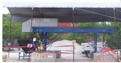
On-line sorting system for separating treated from untreated wood
