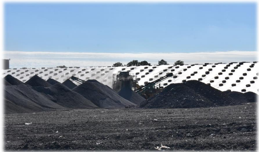
Figure 6-2 Segregated Aggregate Piles
