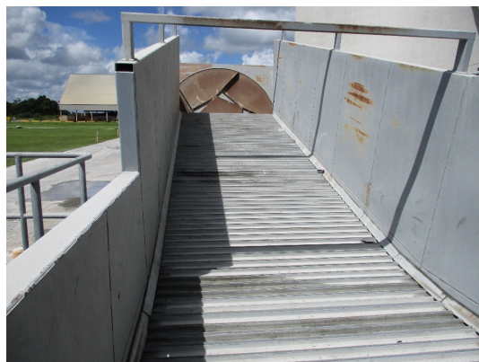
Empty waste tire conveyor belt
