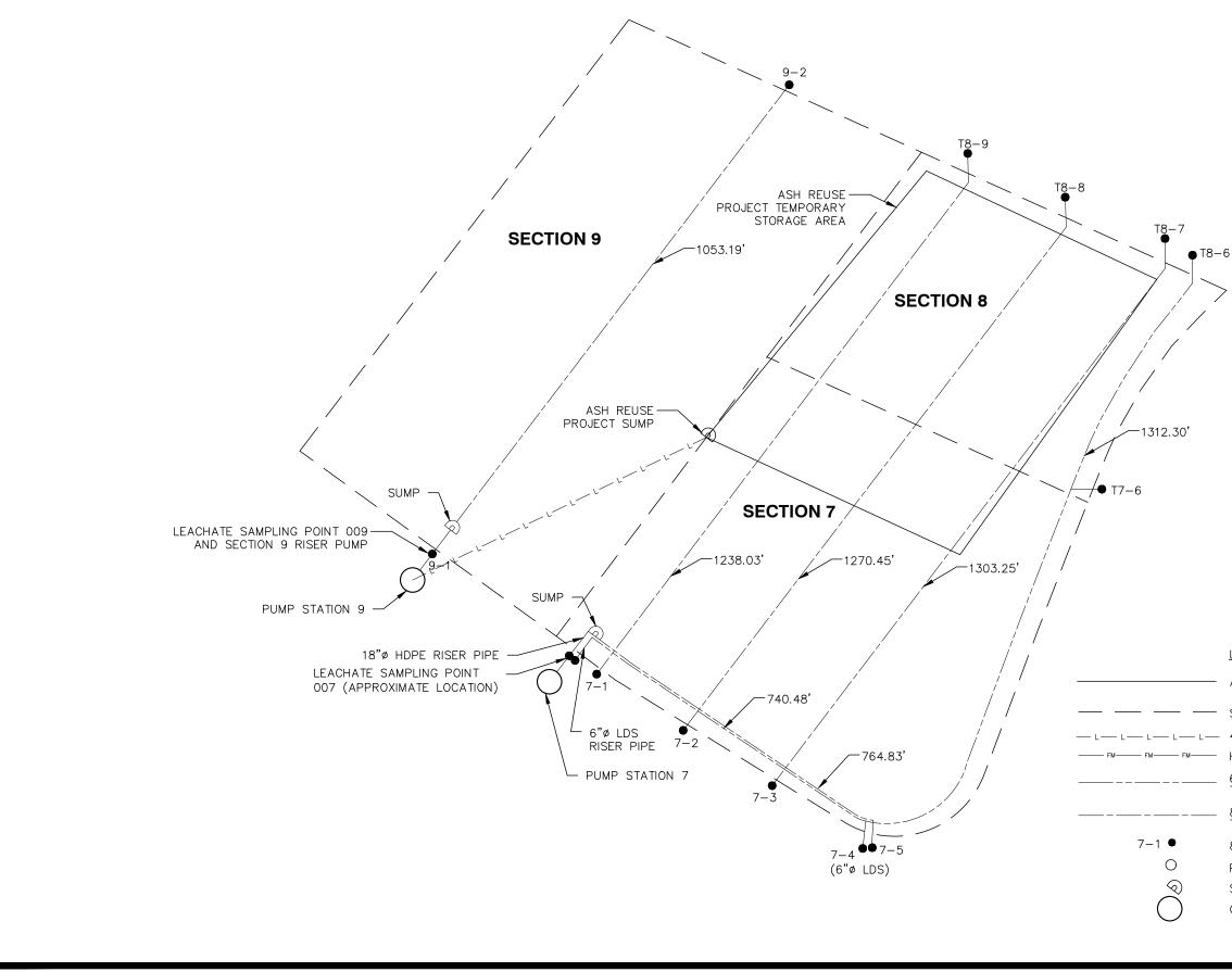
FIGURE 3-2. CAPACITY EXPANSION AREA (SECTIONS 7, 8, AND 9) - LEACHATE COLLECTION AND REMOVAL SYSTEM HILLSBOROUGH COUNTY APRIL 2021
