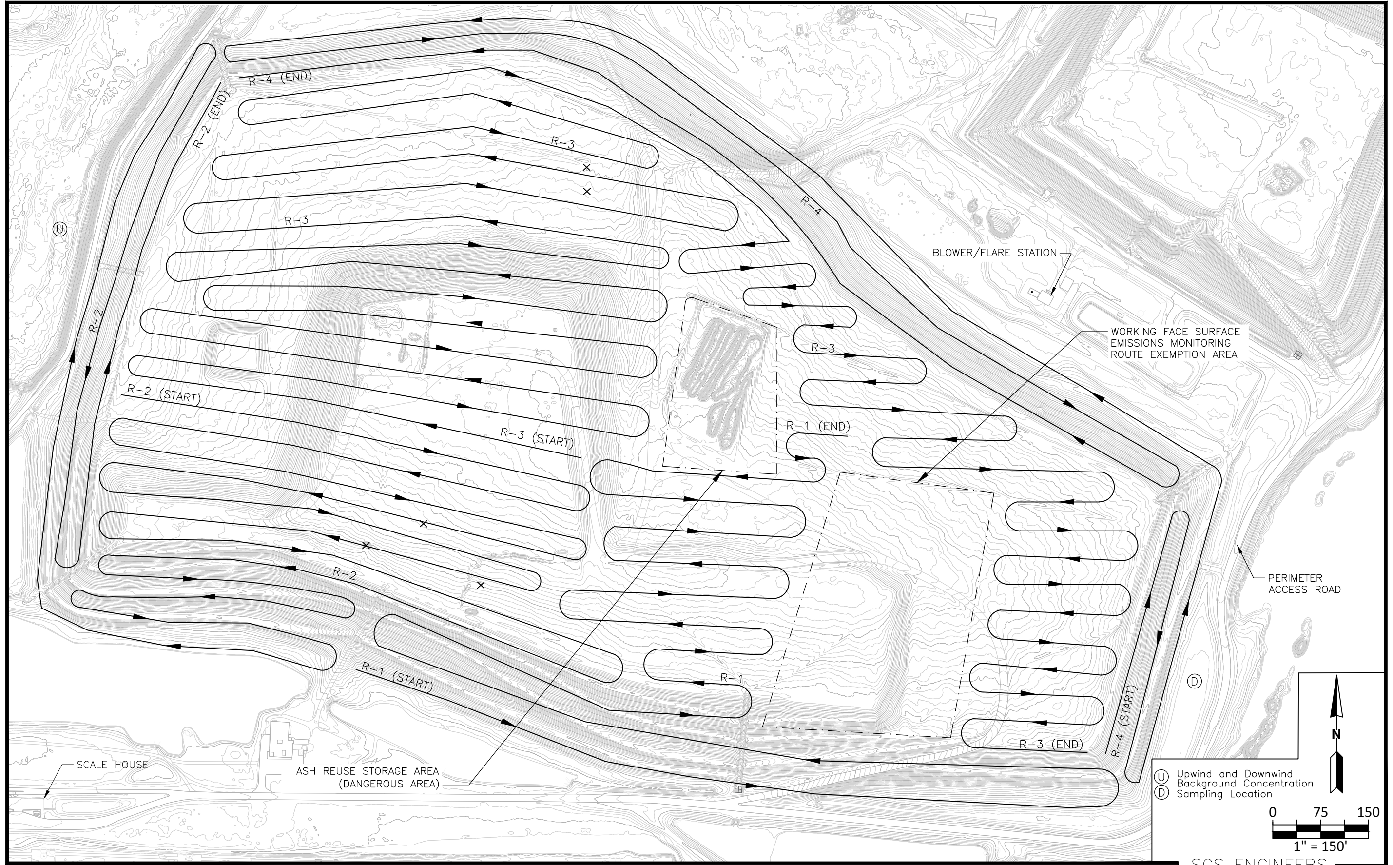
ATTACHMENT 1 - FIGURE 1. 1ST QUARTER 2021 SURFACE EMISSIONS MONITORING PHASES I-VI, SOUTHEAST COUNTY LANDFILL HILLSBOROUGH COUNTY, FLORIDA
