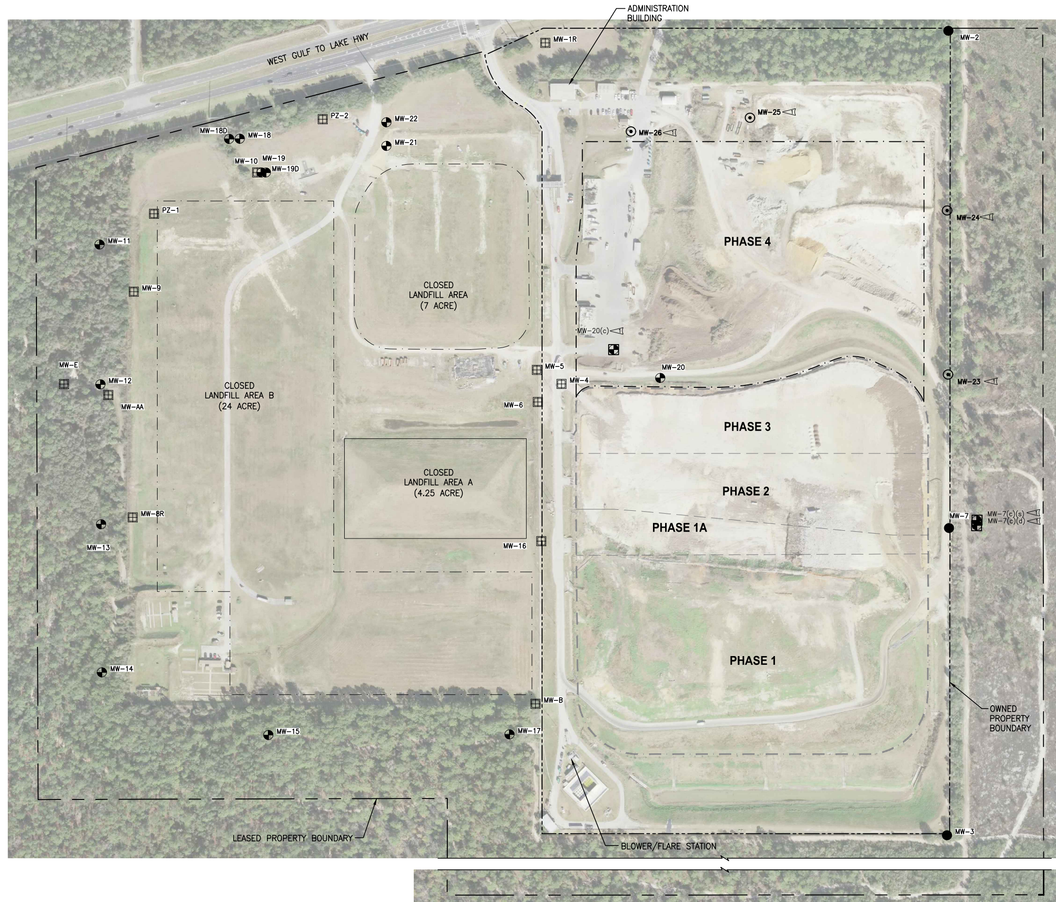
FIGURE L.1 SITE PLAN AND GROUNDWATER MONITORING NETWORK CITRUS COUNTY CENTRAL LANDFILL CITRUS COUNTY, FLORIDA
